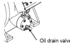
Oil drain valve
